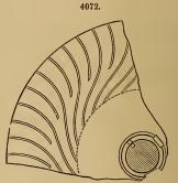
Part of the wheel, Fig. 4071, on a larger scale, to show the form of the vanes more accurately.
